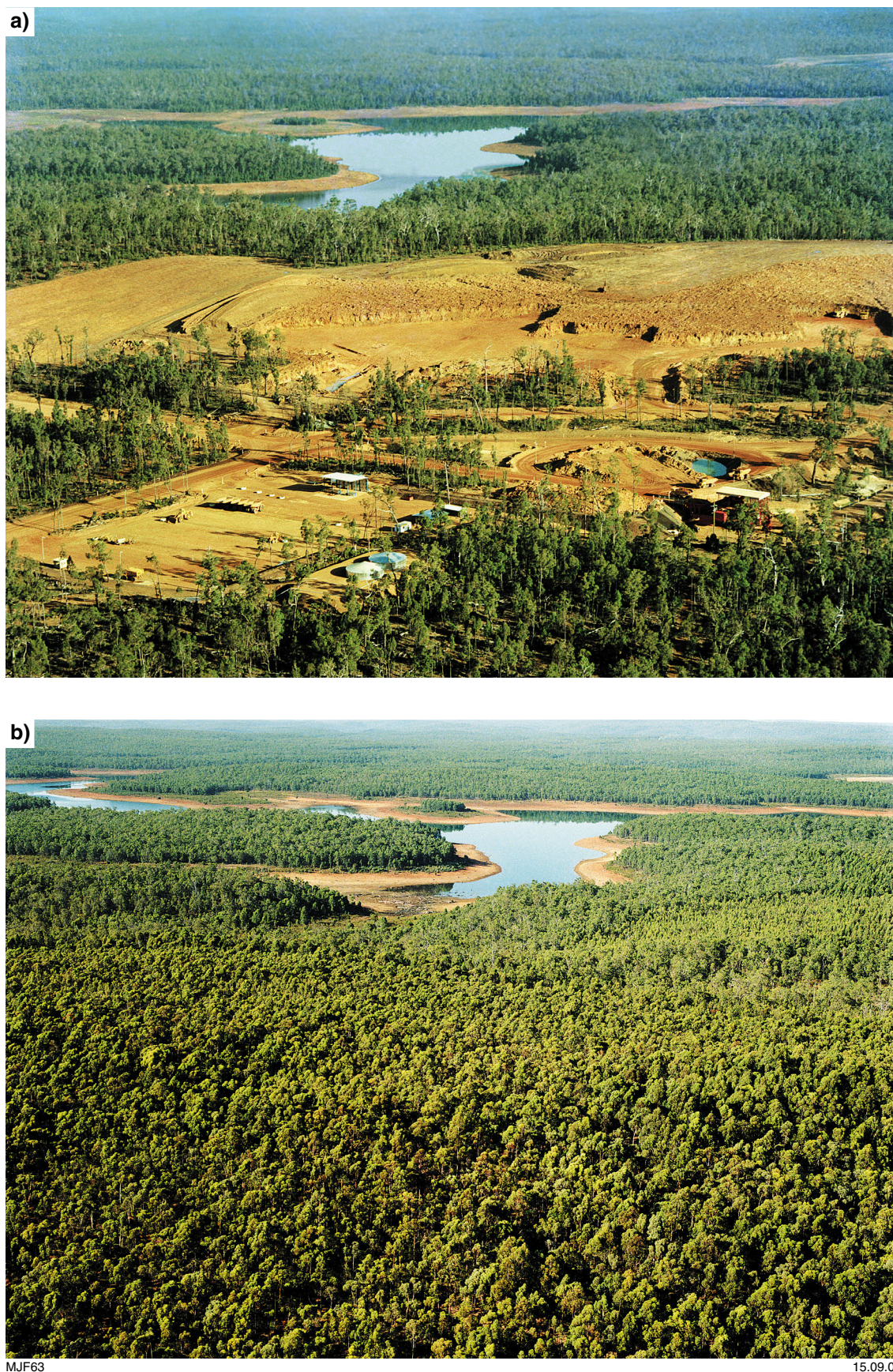
Figure 12. Photographs of mining area at Huntly: a) mobile crushing plant and other mine infrastructure in front of cleared partially mined area, with North Dandalup reservoir beyond; b) same site four years later following rehabilitation of all the cleared areas and restoration of the landforms (photos courtesy of Alcoa World Alumina Australia)
