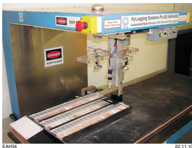
Figure 2. Example of an ASD-based HyLogging system measuring drill chip trays
