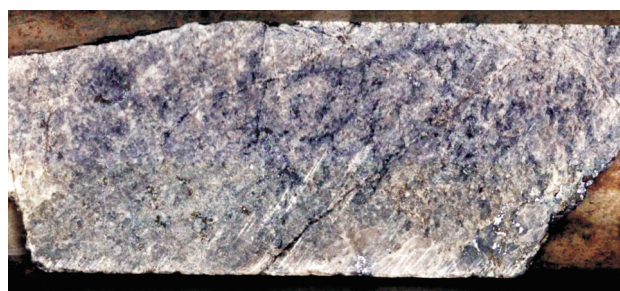
Figure 19. TSG image of Mg-chlorite veinlets in granite from Minnie Springs drillhole MSD1
