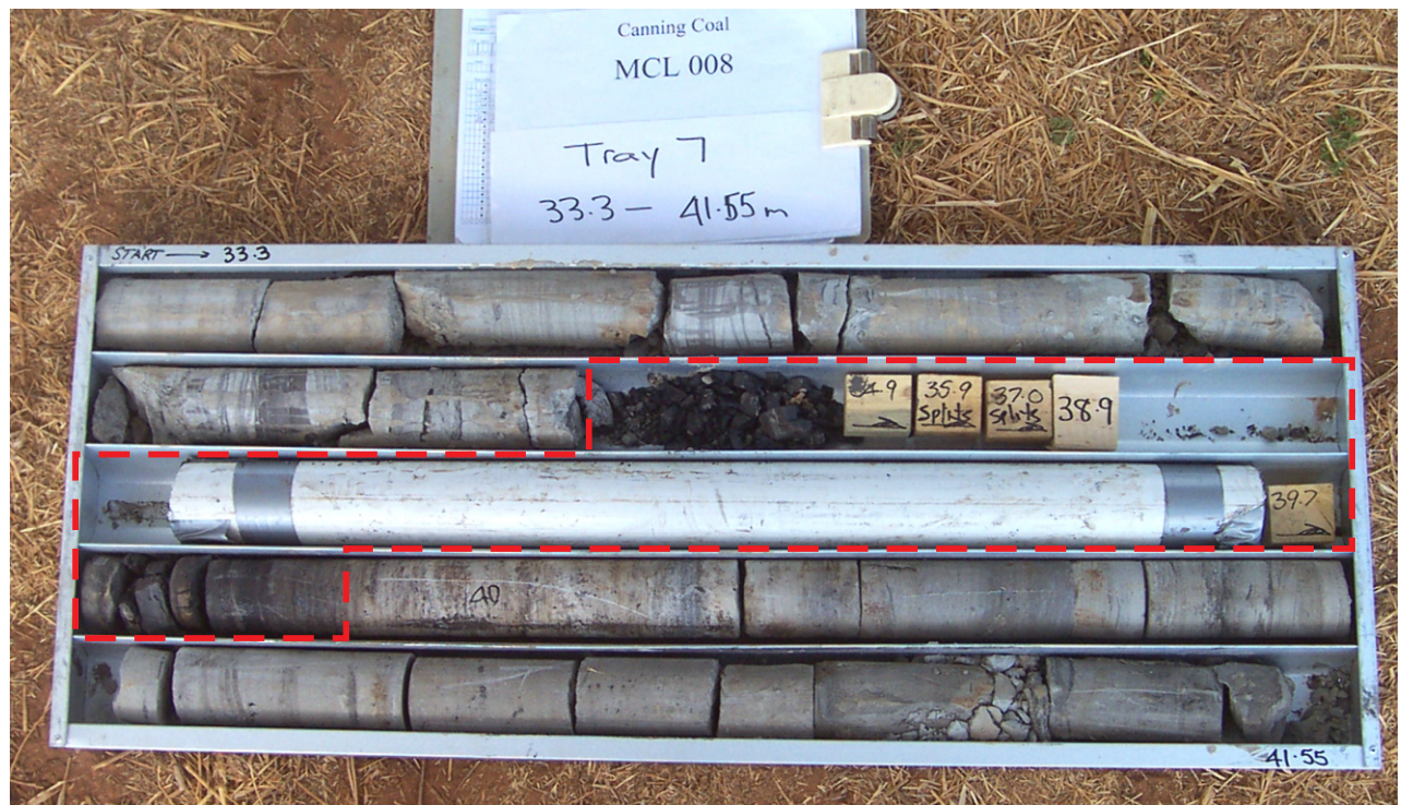
Figure 9. Rio Tinto drillhole MCL008 showing a single, shaley, banded seam that was intersected between 34.8 – 39.8 m and interpreted as seam B (Millar, 2004)
