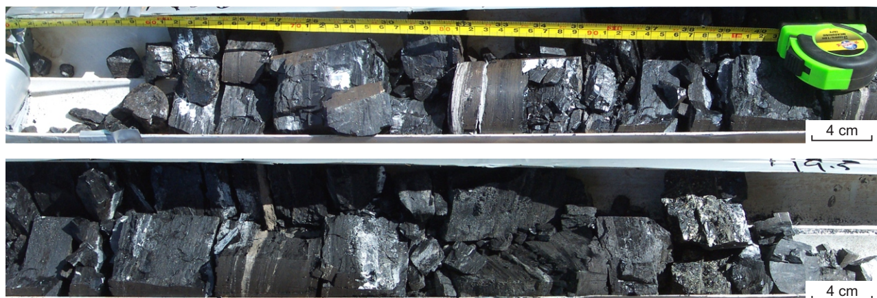
Figure 10. Rio Tinto drillhole PAR001 showing the coal upper (A) seam intersection between 18.6 and 19.5 m (Millar, 2004)
