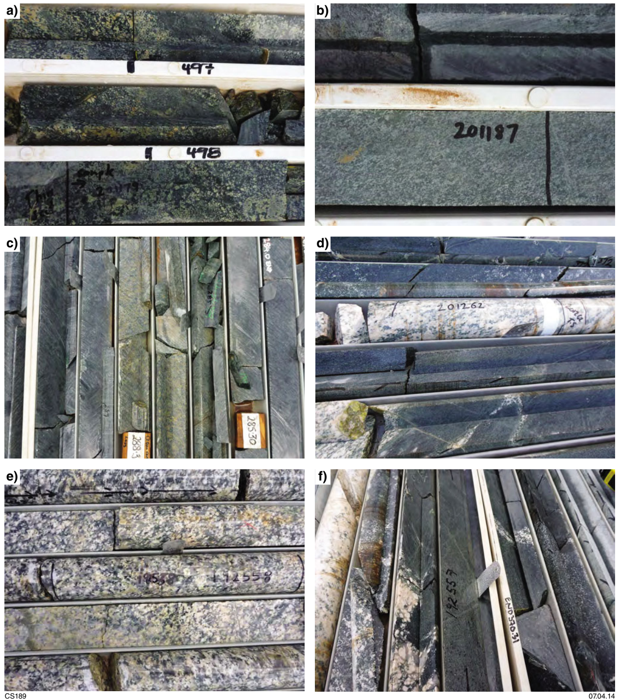
Figure 12. Photographs of drillcore from the Loongana and Haig prospects showing: a) weakly layered medium- to coarse-grained gabbro from Haig (HDDH001); b) fine- to medium-grained gabbro from Haig (HDDH001); c) medium-grained gabbro, including a layer of cumulate-textured olivine-rich gabbro (brown-stained rock), from Loongana (LNGD001); d) plagiogranite intrusions within fine- to medium-grained gabbro from Loongana (LNGD001); e) dated tonalitic gneiss sample GSWA 192558 in Loongana core (LNGD002); f) dated metagabbro sample GSWA 192557 in Loongana core (LNGD002).
