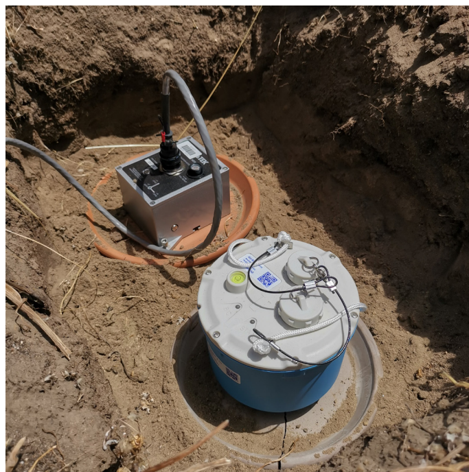
Figure 1. A typical installation for evaluation of seismic risk includes a seismometer (front) and an accelerometer (back) to accurately record seismic waves and ground shaking caused by earthquakes
