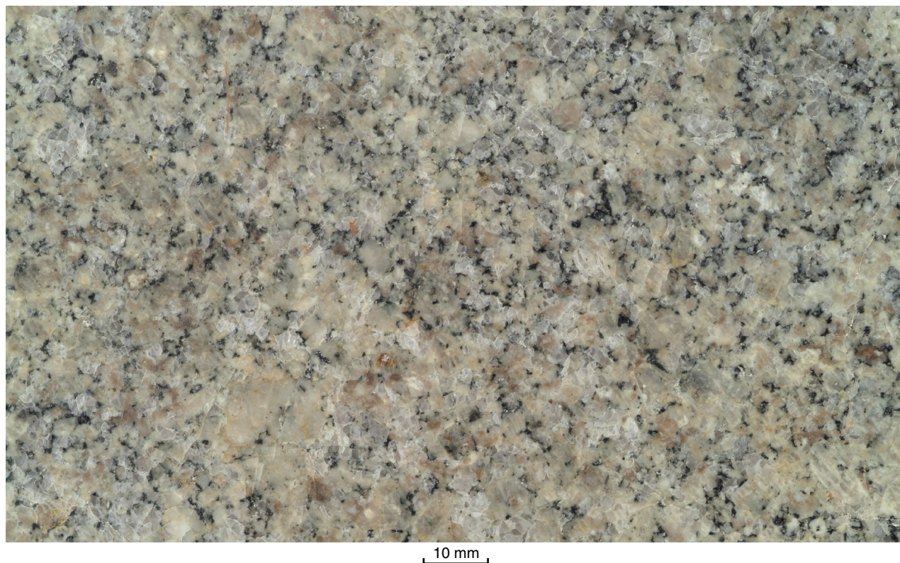
Appendix 3.6. Greenmount granite: weakly deformed monzogranite, Greenmount Hill quarry
