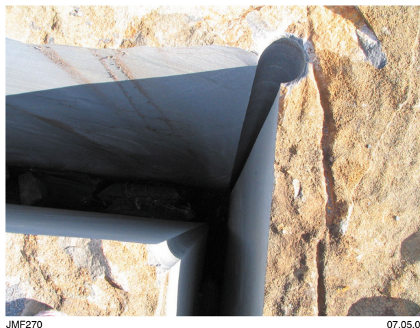
Figure 39. Vertically drilled, 30 mm pilot hole at top into which the diamond wire is threaded. Note the smooth, vertical faces resulting from the diamond wire cutting process. Orange Grove black granite, Bridgetown
