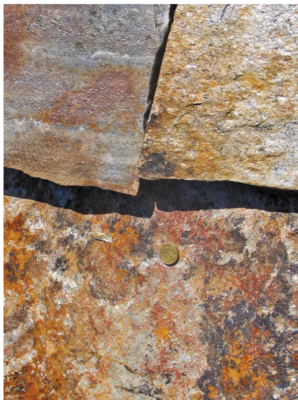
Figure 129. A selection of more schistose, quartzitic forms of Toodyay Stone from the Black and Tan quarry ranging in colour from pale red-brown, medium brown, to dark brown
