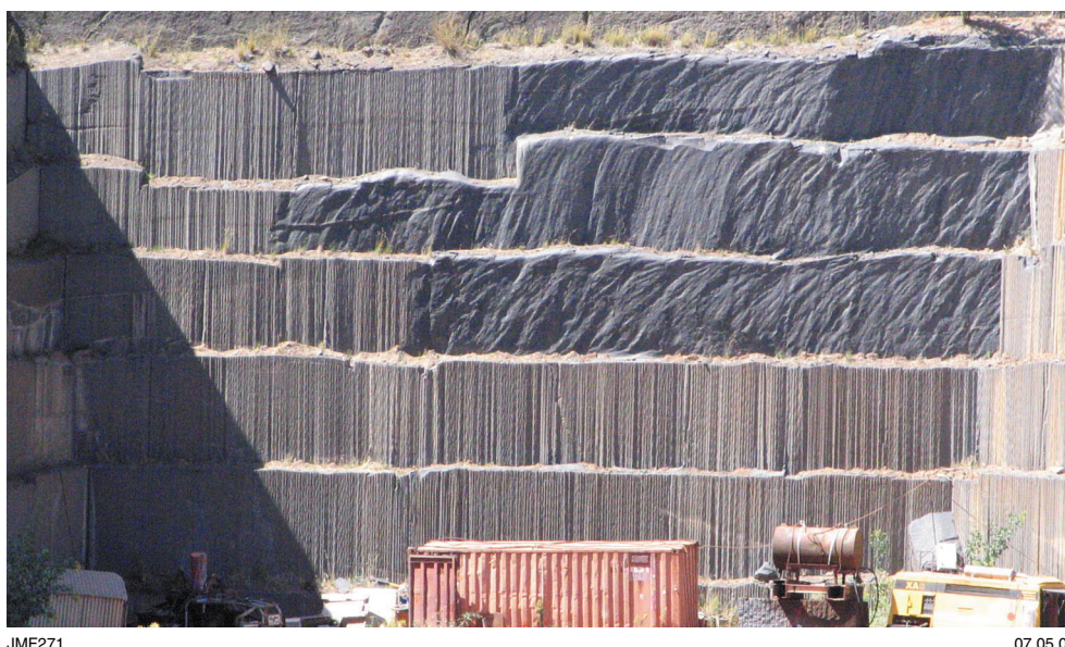
Figure 41. Blackened quarry walls at upper right previously subjected to thermal lance cutting
