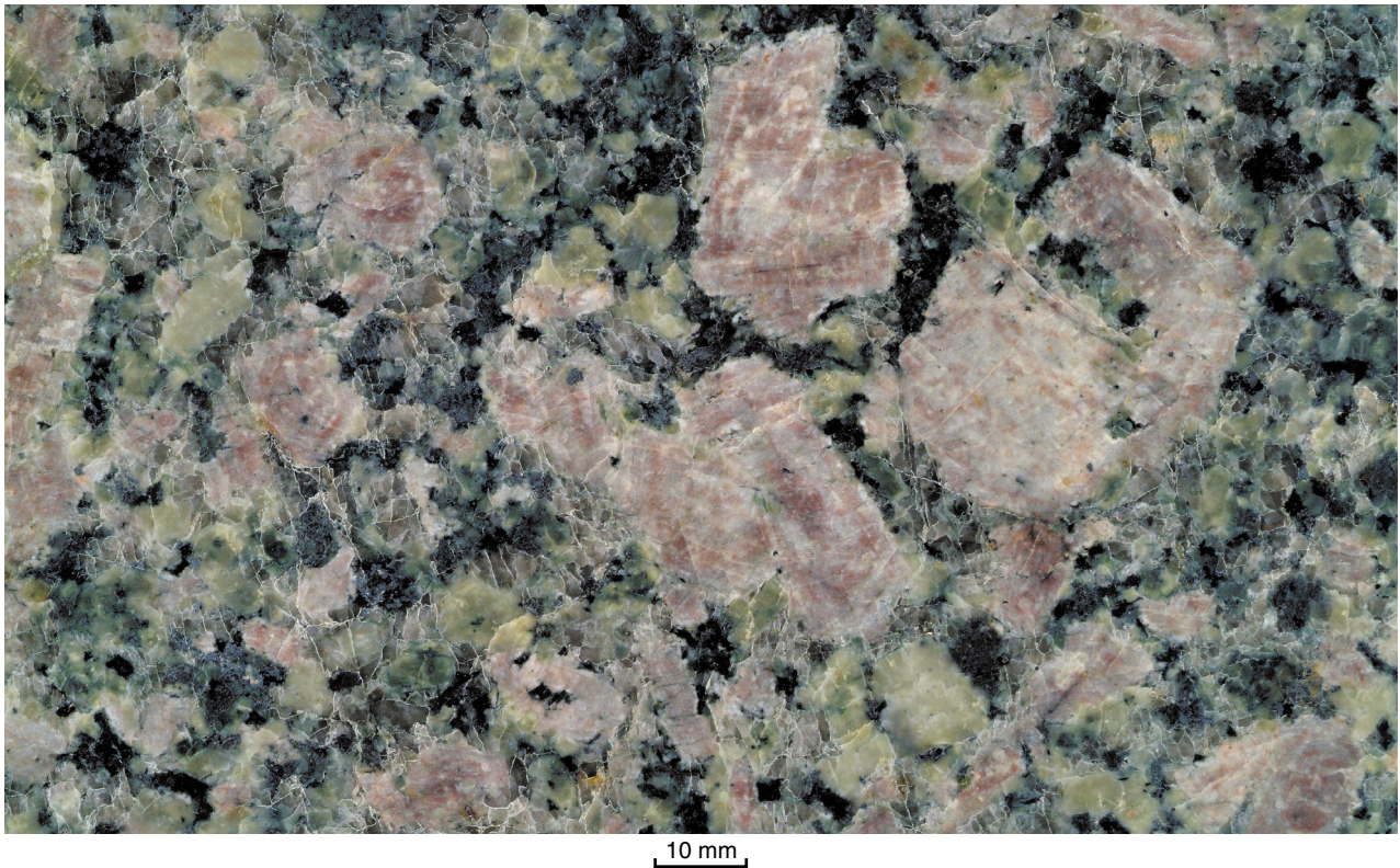
Appendix 3.15. Valmere Green granite: coarse-grained, heterogeneous, quartz monzonite, Watheroo
