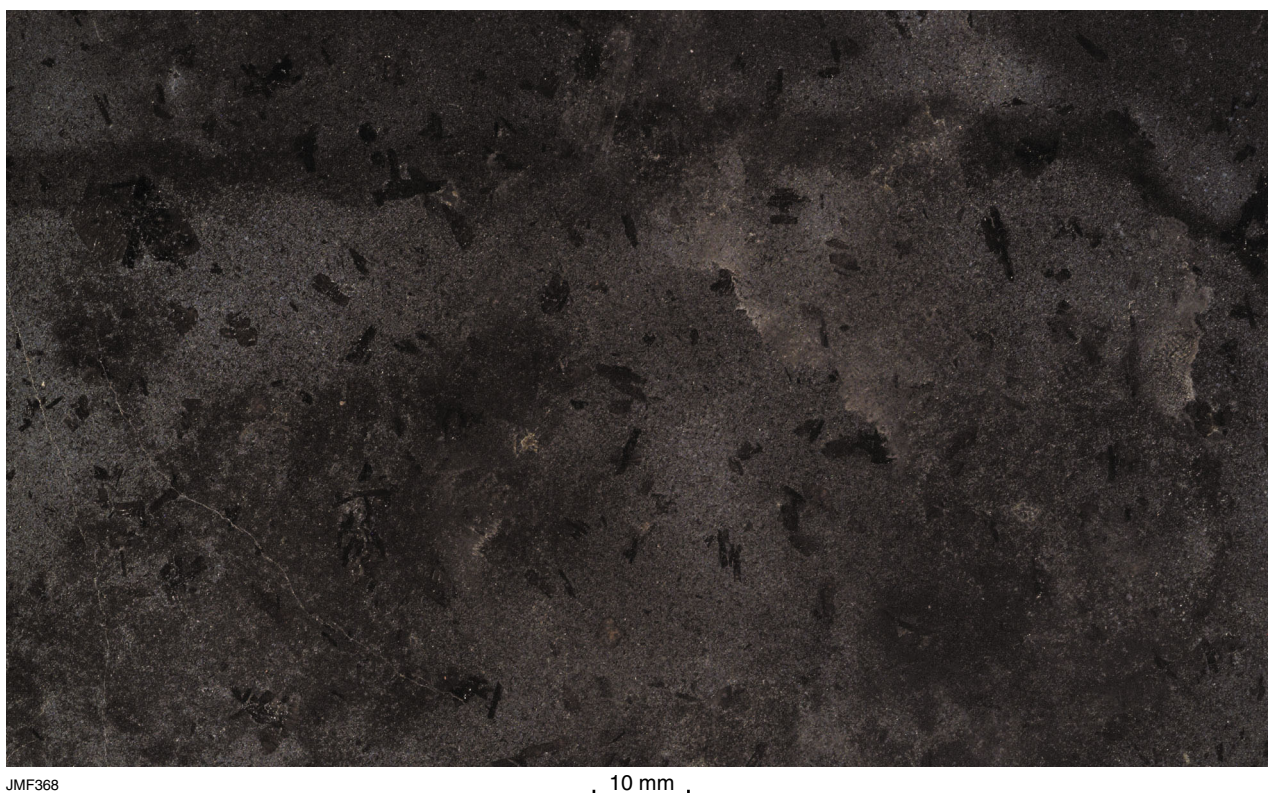
Appendix 3.28. Bunbury Basalt: dark grey porphyritic basalt, Jules Road quarry, Gelorup
