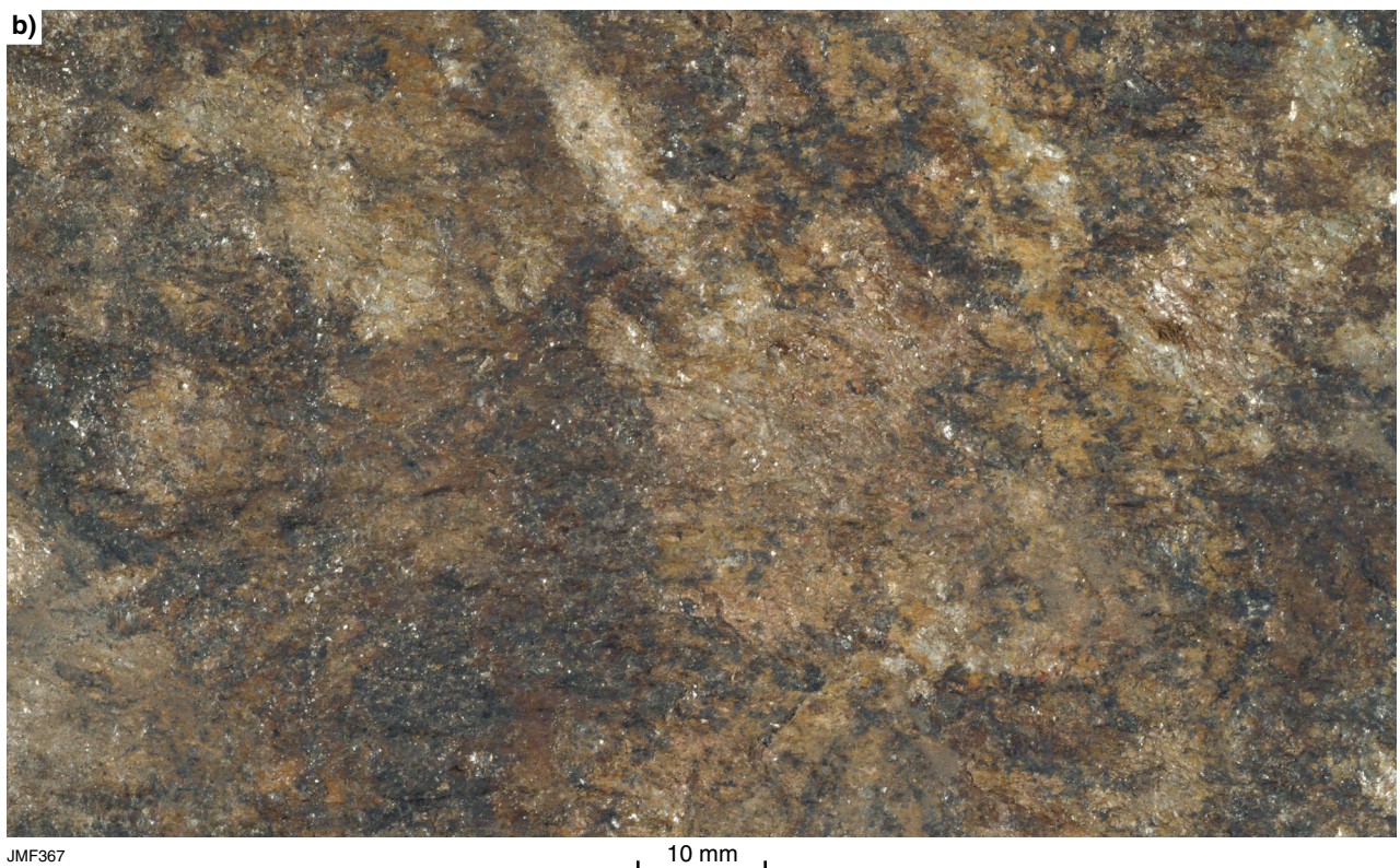
Appendix 3.26. Toodyay Stone: schistose, medium-grained metasandstone: a) mid-brown variety with pale green fuchsite patches on parting plane; b) variegated, mid- to dark brown variety, Black and Tan quarry, Toodyay
