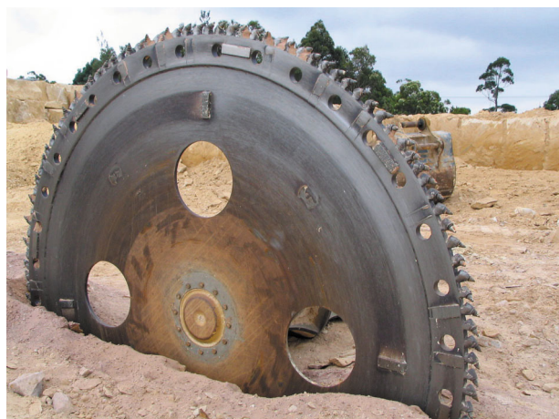
Figure 49. A 3 m-diameter cutting wheel fitted with tungsten carbide cutting picks for cutting relatively soft sandstone
