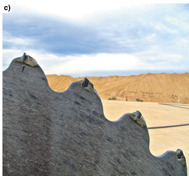
Figure 51. Extractive process for limestone (calcarenite) building blocks: a) The level limestone floor is cut with a series of parallel saw cuts to produce blocks in a variety of standard sizes; b) rail-mounted, multi-blade quarry saw cutting standard size blocks; c) quarry saw blade fitted with tungsten carbide cutting teeth; d) quarry-cut blocks packed on site for dispatch to clients (photo (d) courtesy Meteor Stone)
