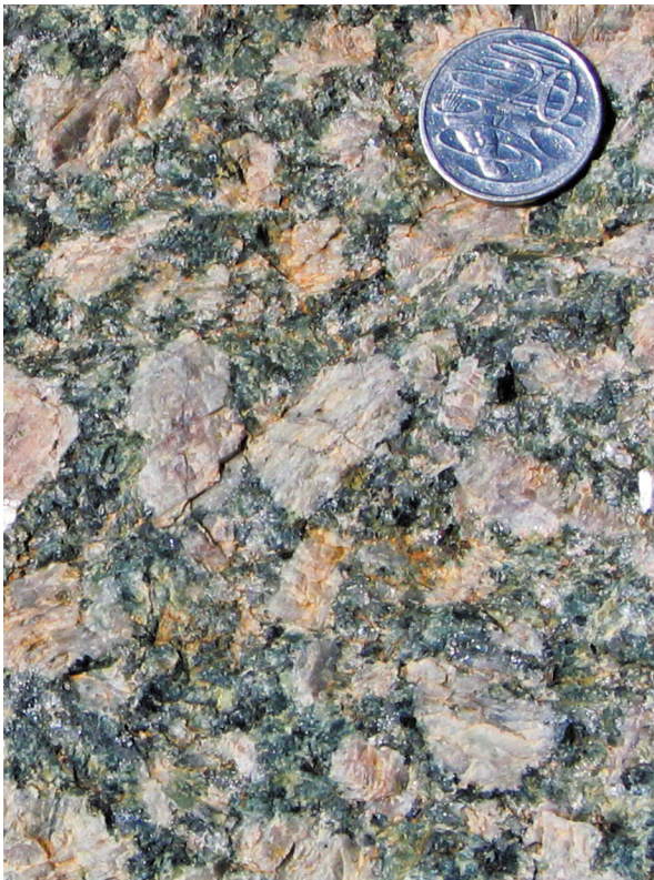
Figure 108. The coarse-grained Valmere Green quartz monzonite in hand specimen
