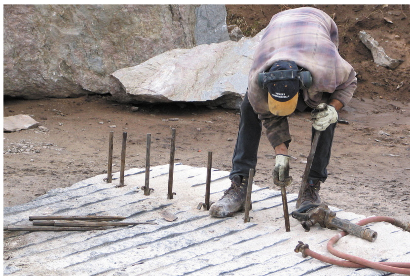
Figure 44. A quarryman inserting sets of plug and feathers in a line of drillholes
