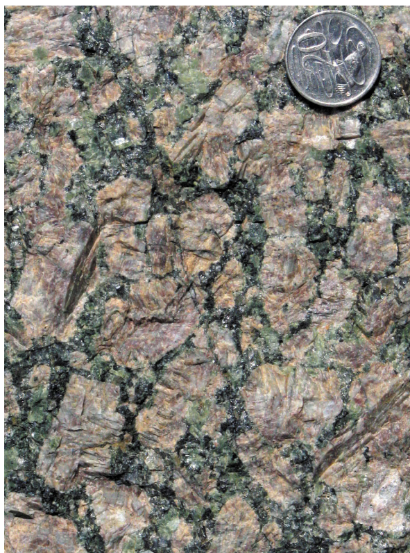
Figure 112. The very coarse grained Mulroy Green monzogranite containing large green masses of plagioclase grains interspersed between deep pink K-feldspar megacrysts
