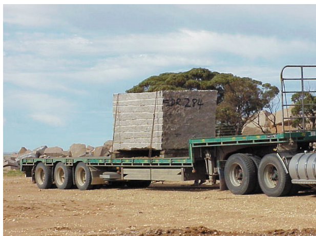
Figure 48. Low loader transporting a 10 tonne block of Esperance granite (photo courtesy Melocco Stone)
