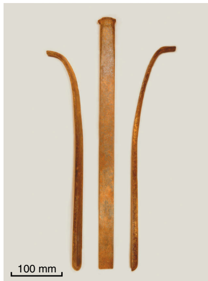
Figure 43. A set of plug and feathers used for final block splitting
