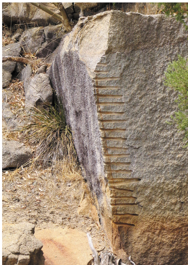
Figure 95. Original granite working face still present in the Mundaring quarry. Note the old plug and feather holes used to cleanly split block faces
