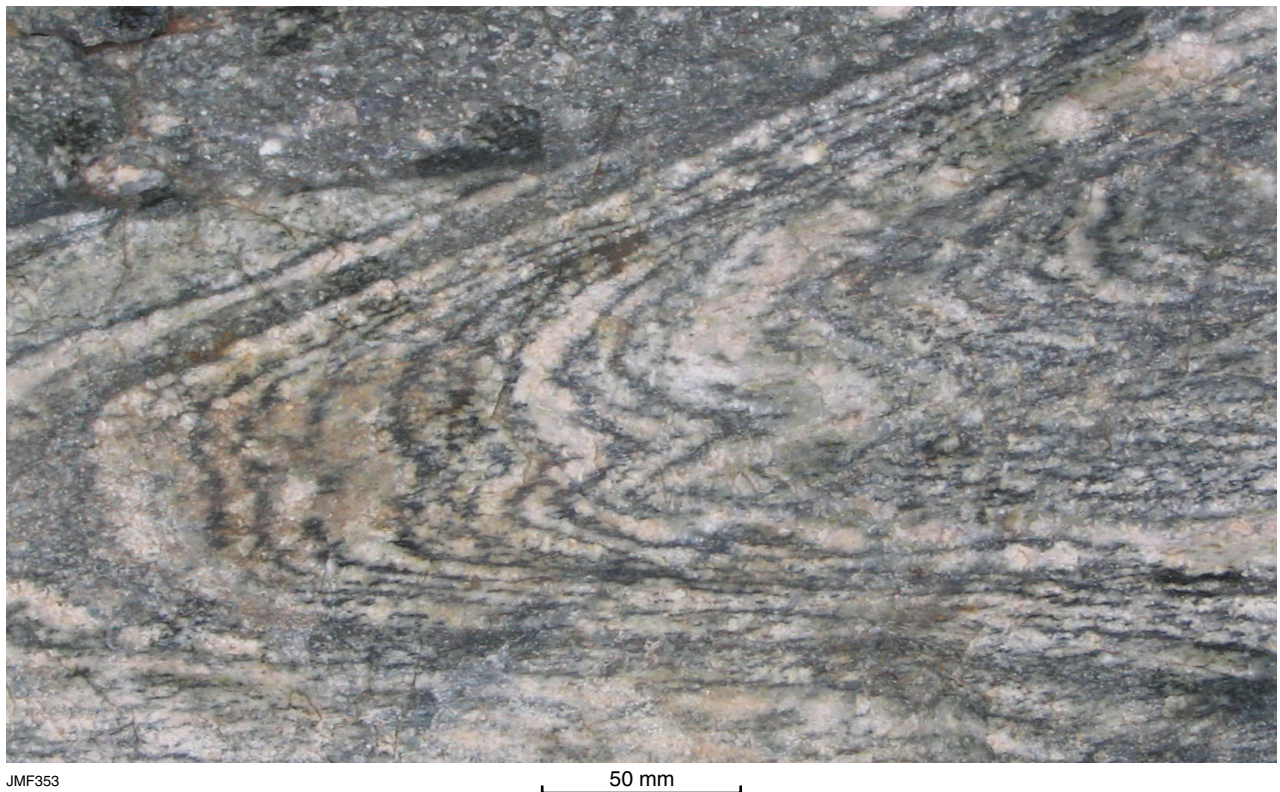
Appendix 3.5. Carrido Spring gneiss: gneissic tonalite, Carrido Spring quarry
