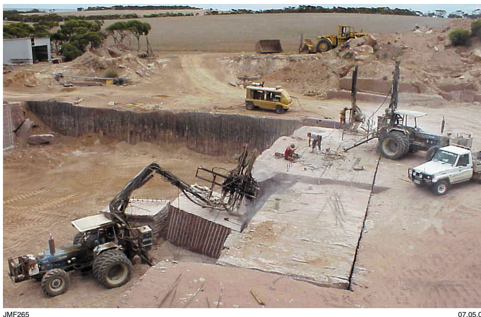
Figure 34. An 800 t primary block of Desert Brown granite from Esperance in the far south of Western Australia. The primary block, previously separated by close-spaced drilling and diamond wire sawing, is being subdivided into secondary blocks by in-line drilling (centre right). At centre left, an in-line block drill is cutting a smaller, tertiary block into saleable-sized blocks (photo courtesy Melocco Stone)
