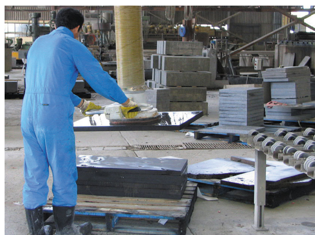
Figure 53. A vacuum cup hoist in operation transporting polished basalt slabs
