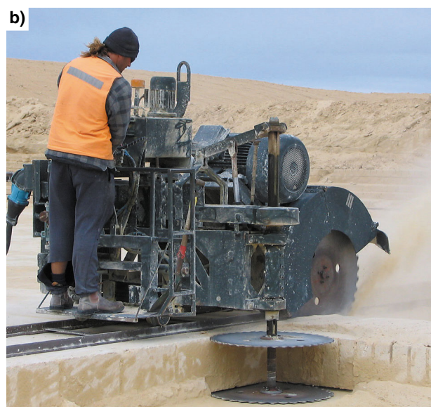
Figure 50. Sandstone block sawing operations. A 3.5 m-diameter rock saw, mounted on the arm of an excavator, deftly cuts out sandstone blocks
