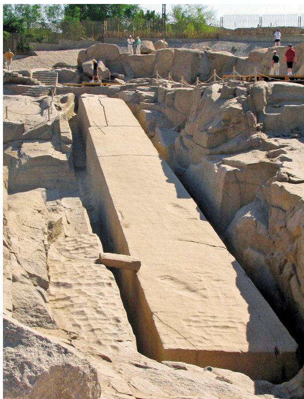
Figure 5. Unfinished, 42 m-tall obelisk (1450 BC) in situ in the Aswan granite stone quarry in southern Egypt. Note the shallow slots cut in the rock (left foreground). It is thought wooden wedges were forced into these slots beneath a newly completed block causing the block to split away from the quarry floor (Glover, 2003)
