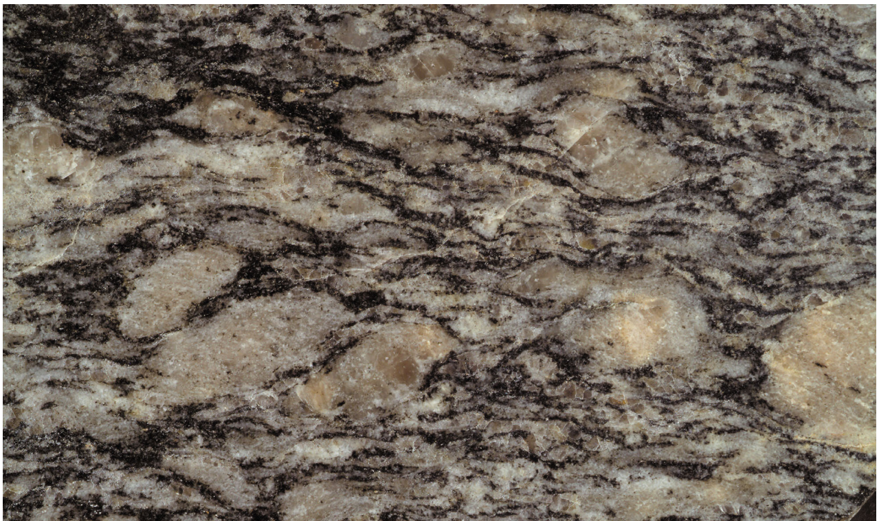
Appendix 3.14. Roelands gneiss: heterogeneous biotite monzogranite gneiss, Roelands quarry
