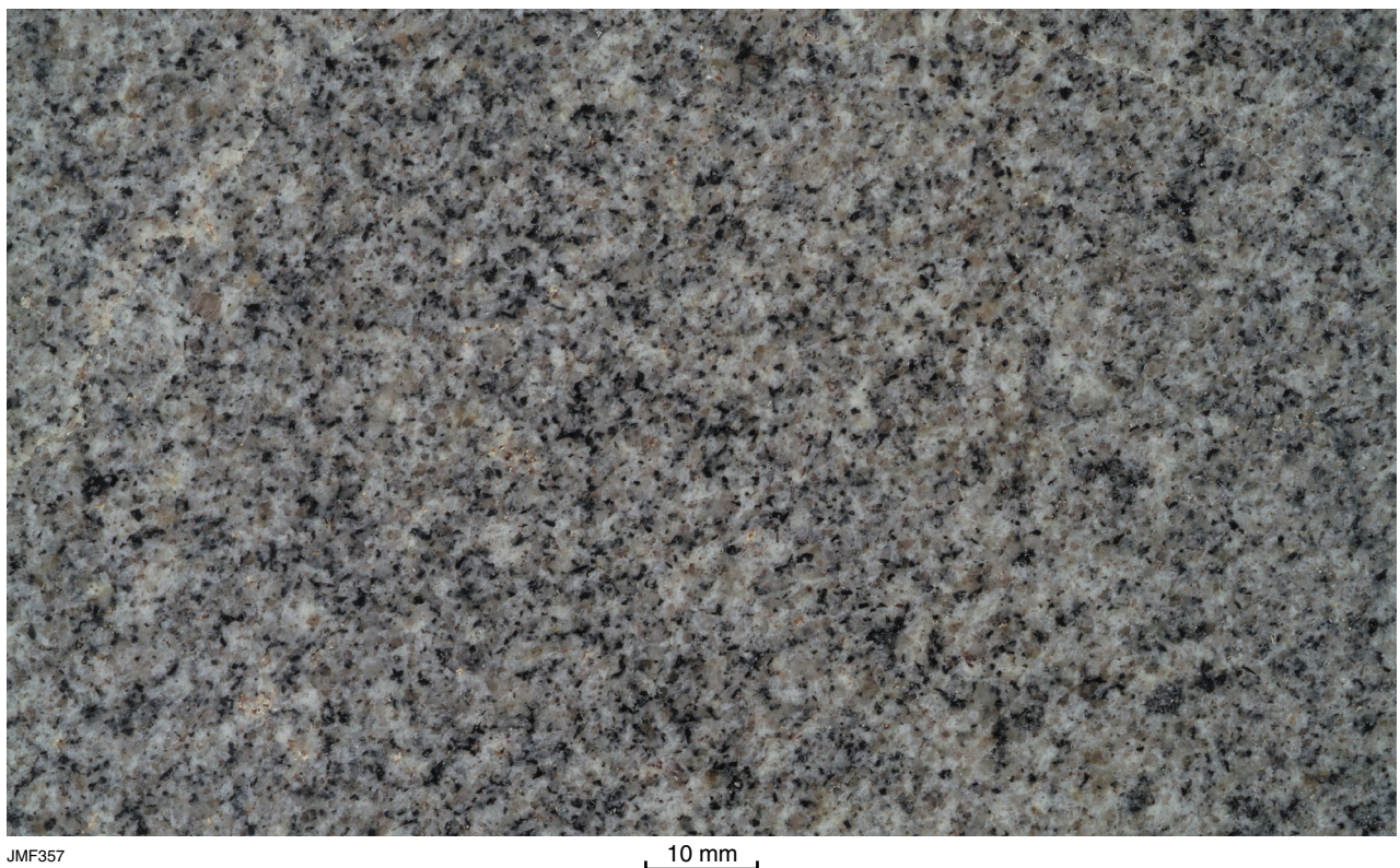
Appendix 3.11. Meckering granite: fine-grained, grey, uniform, biotite-quartz monzodiorite, Meckering quarry
