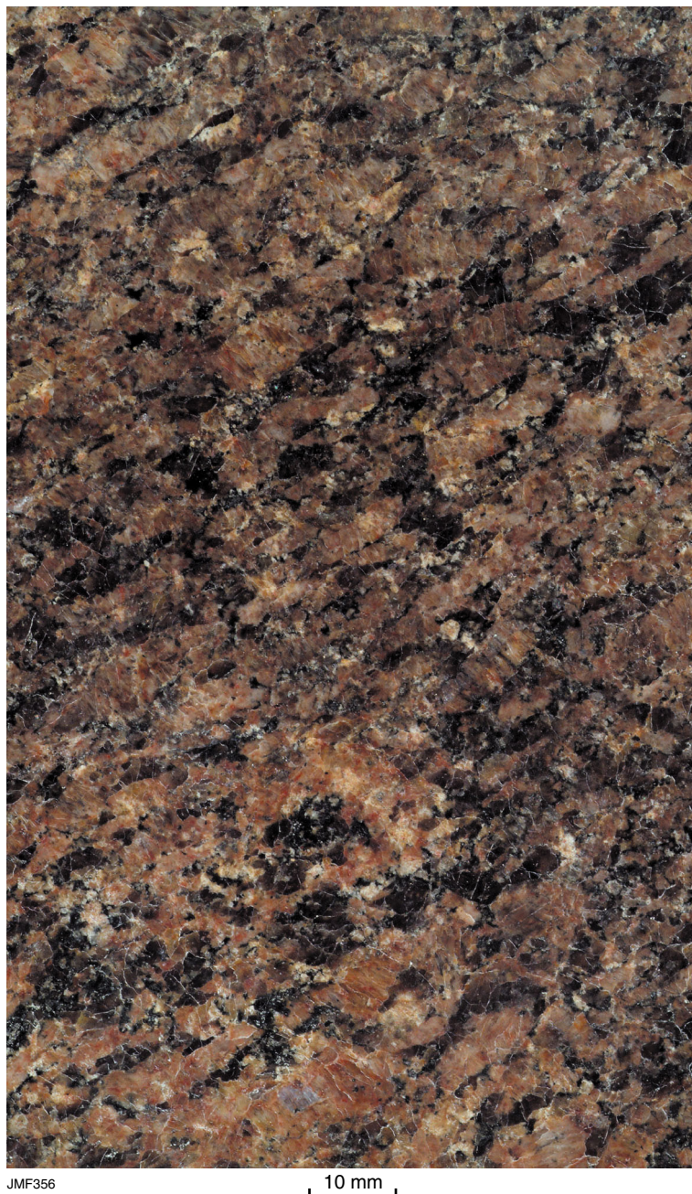
Appendix 3.9. Karlgarin granite gneiss: biotite syenogranite gneiss, Karlgarin quarry
