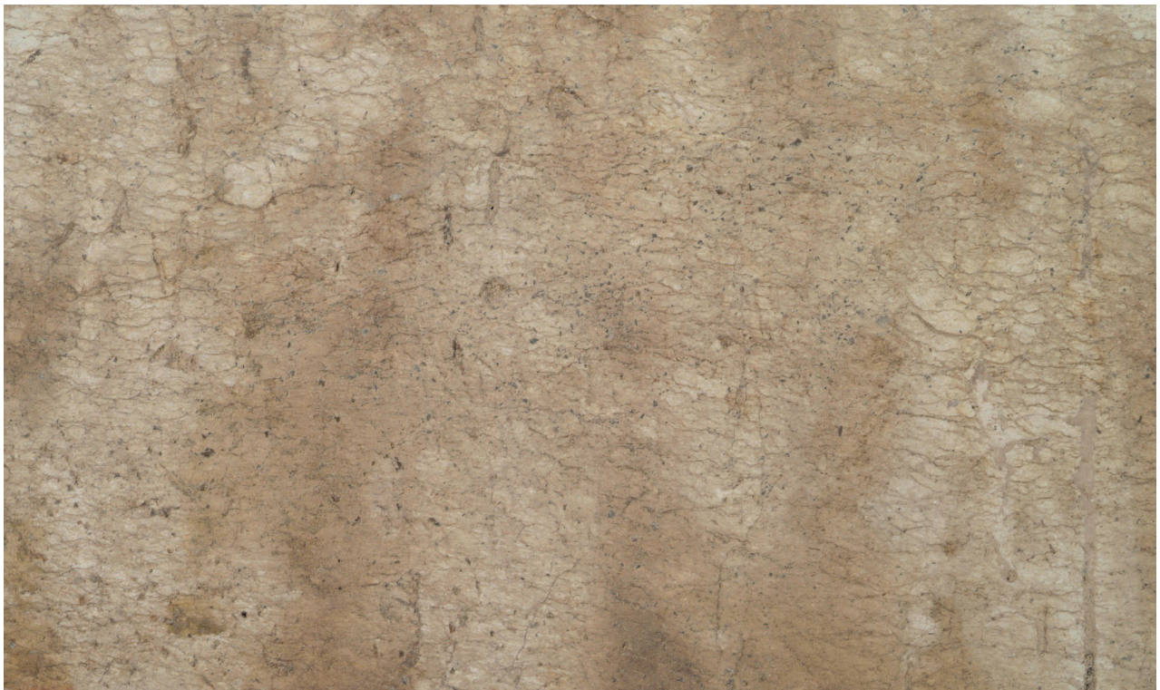
Appendix 3.32. Casuarina Stone : massive to weakly layered diatomite, predominantly composed of silty claystone, Gingin Brook environs, Gingin
