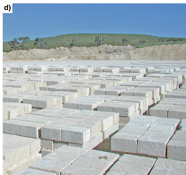
Figure 51. Extractive process for limestone (calcarenite) building blocks: a) The level limestone floor is cut with a series of parallel saw cuts to produce blocks in a variety of standard sizes; b) rail-mounted, multi-blade quarry saw cutting standard size blocks; c) quarry saw blade fitted with tungsten carbide cutting teeth; d) quarry-cut blocks packed on site for dispatch to clients (photo (d) courtesy Meteor Stone)
