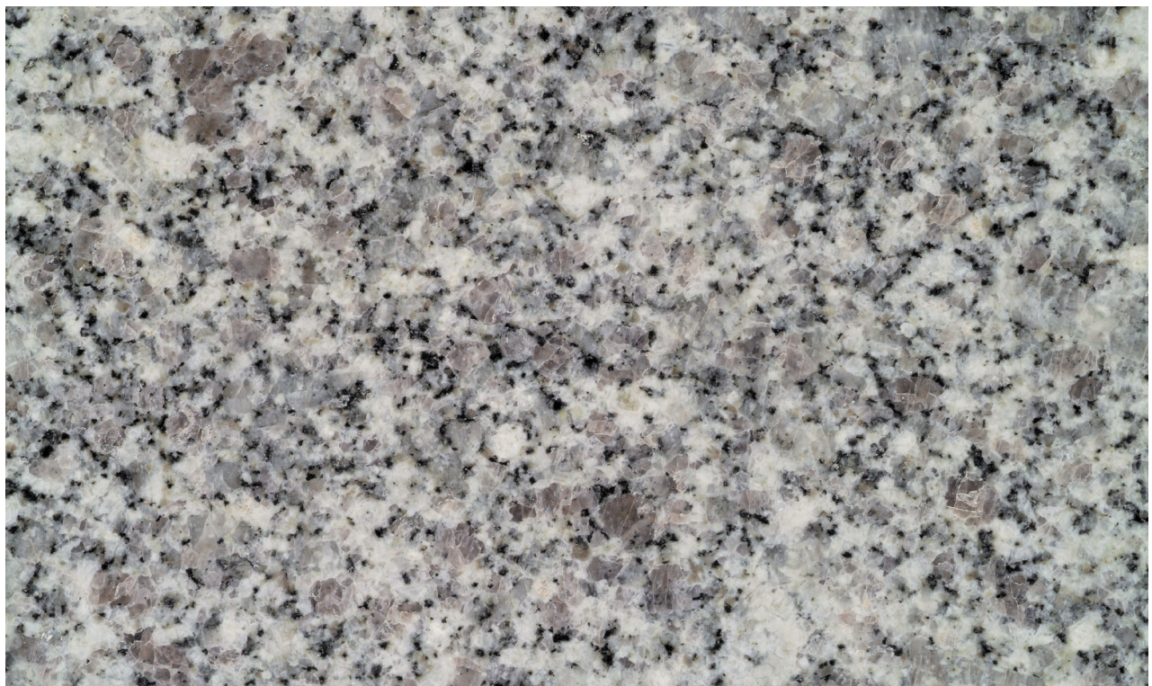
Appendix 3.8. Mundaring granite: inequigranular monzogranite, Mundaring quarry
