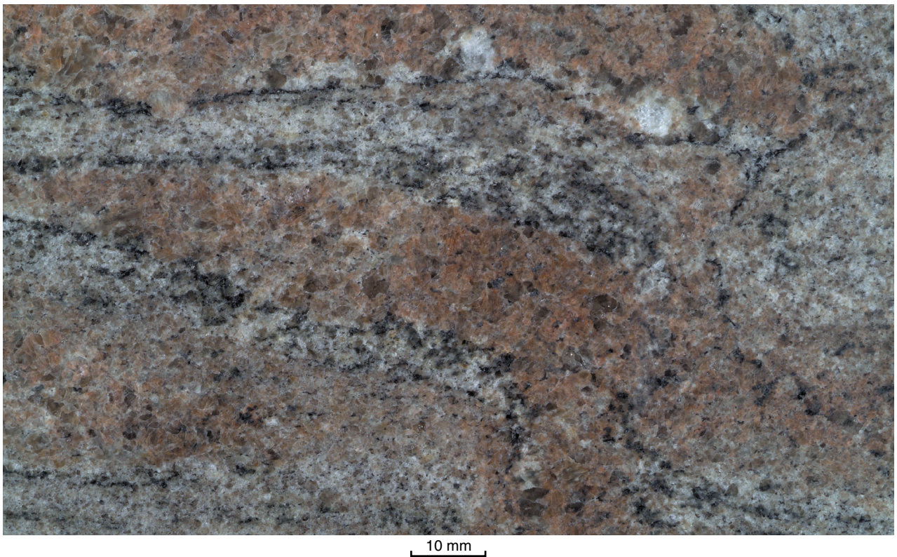
Appendix 3.2. Austral Waterfall : leucocratic quartz monzonite granofels, Bruce Rock
