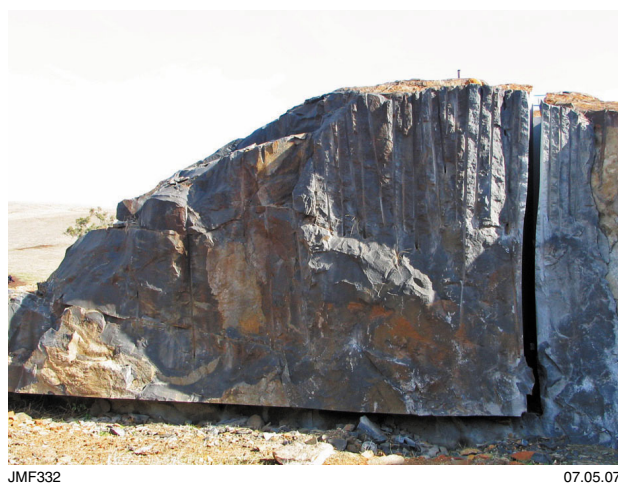
Figure 120. Diamond wire-sawn primary black granite block at Orange Grove quarry
