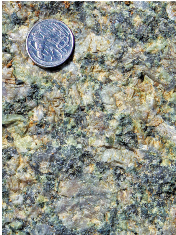
Figure 109. Coarse-grained, megacrystic, hornblende-biotite Verde Lope monzogranite
