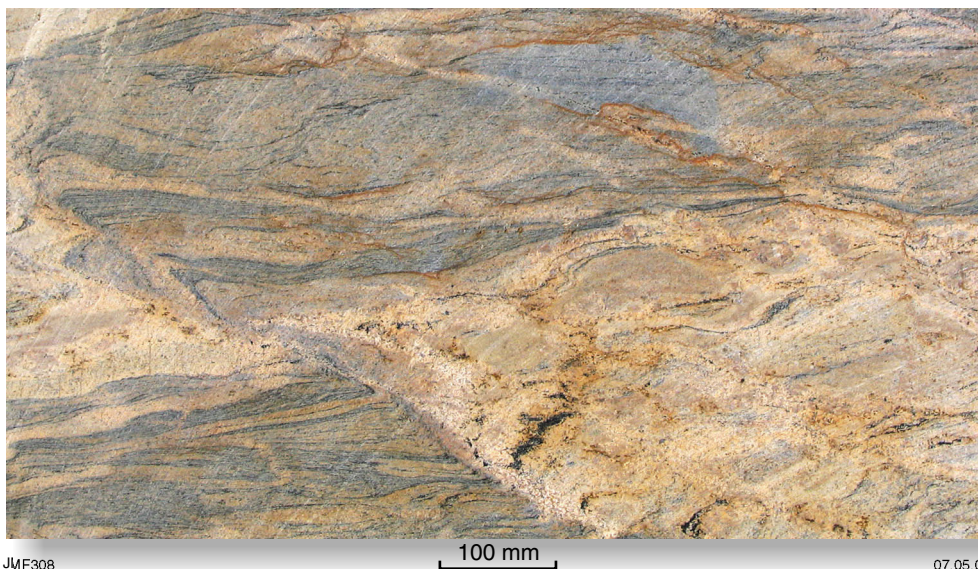
Figure 85. Diamond wire-cut face of an Austral Juperana block illustrating the visually attractive swirling texture present throughout the stone
