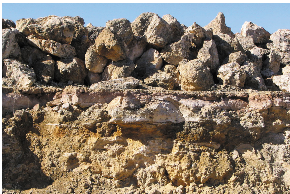
Figure 144. Tamala Limestone near-surface, 'capstone' profile, Hope Valley–Postans area. Photo shows the upper, hard 'capstone' layer, about 0.5 m thick, overlying friable, light brown, calcareous sand containing numerous limestone pebble and cobble-sized clasts. Previously ripped capstone boulders, 1.0 to 1.5 m in diameter, are stockpiled at surface
