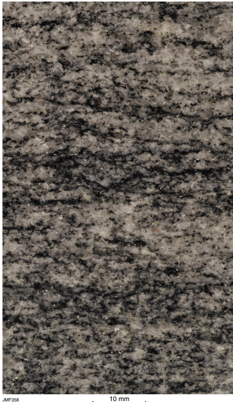
Appendix 3.12. Roelands gneiss: layered biotite monzogranite gneiss, Roelands quarry
