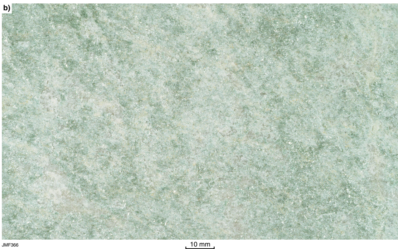
Appendix 3.25. Toodyay Stone: a) silver-grey, coarse-grained quartzite; b) coarse-grained quartzite with pale green fuchsite mica coatings on parting planes, Salt Valley Road quarry, Toodyay
