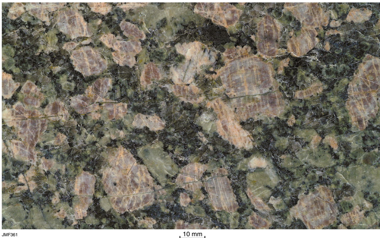
Appendix 3.18. Mulroy Green granite: coarse-grained monzogranite, Namban
