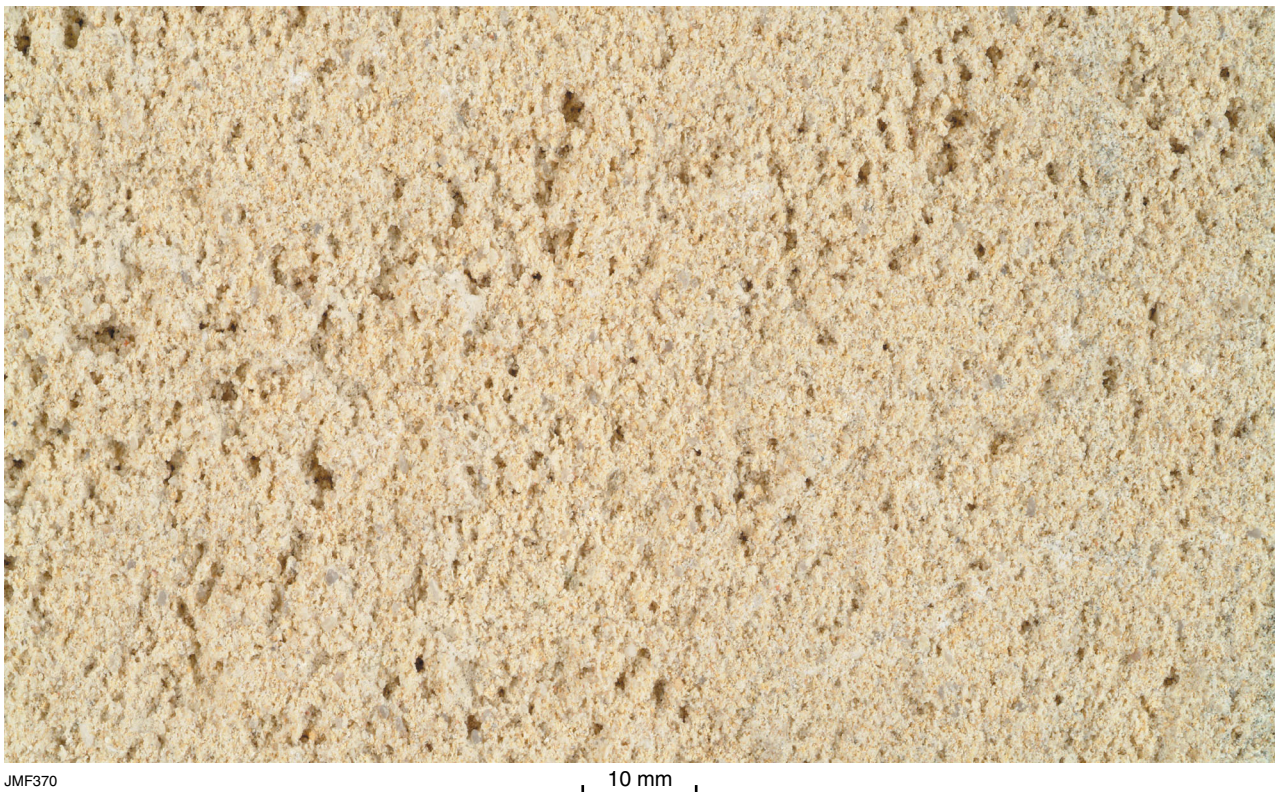
Appendix 3.31. Tamala Limestone: biscuit-coloured, massive, very porous, microfossiliferous building block limestone, Moore River quarry, near Guilderton
