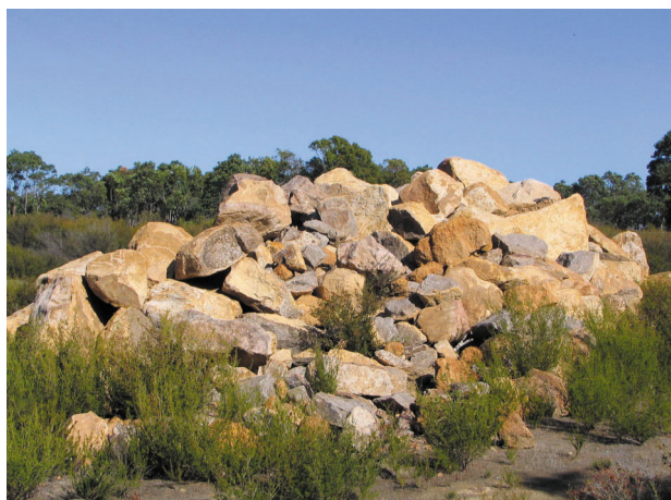
Figure 31. A stockpile of durable granite-gneiss boulders (mostly 2–3 m in diameter) possibly suitable for use as armourstone in breakwater or dam construction. Woodlands granitic gneiss
