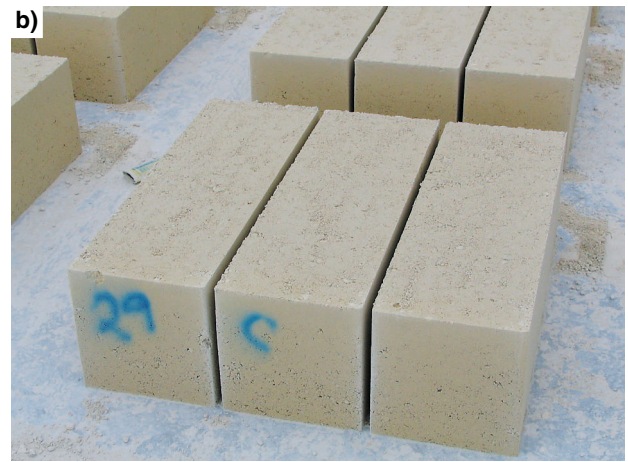
Figure 69. Batch making reconstituted limestone blocks: a) a mobile batching machine in operation; b) a newly formed set of reconstituted blocks, 1.0 m in length
