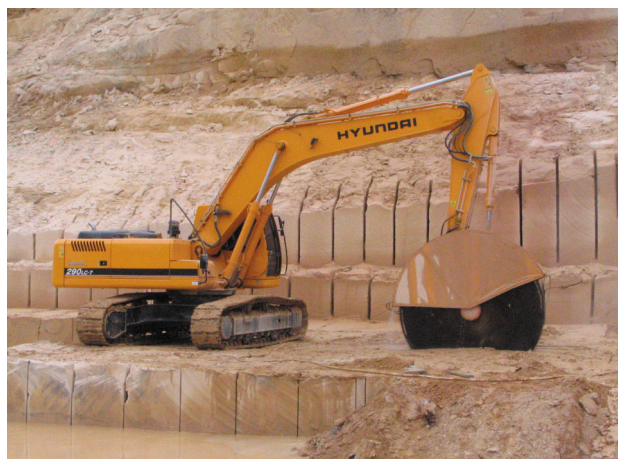
Figure 50. Sandstone block sawing operations. A 3.5 m-diameter rock saw, mounted on the arm of an excavator, deftly cuts out sandstone blocks
