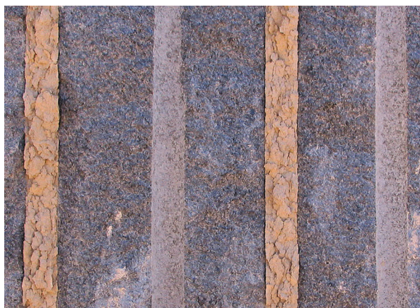
Figure 45. An expanding compound used to effect a clean break along a line of drillholes in black granite. Note the dried expanding material placed in alternate drillholes 250 mm apart
