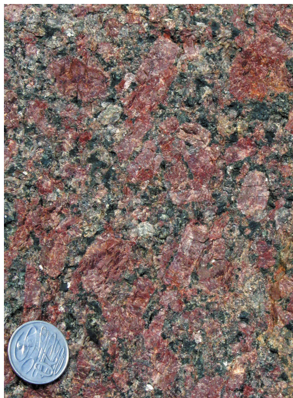
Figure 114. Quarry specimen of Namban Red quartz syenite displaying large, deep red, flow-oriented, K-feldspar crystals
