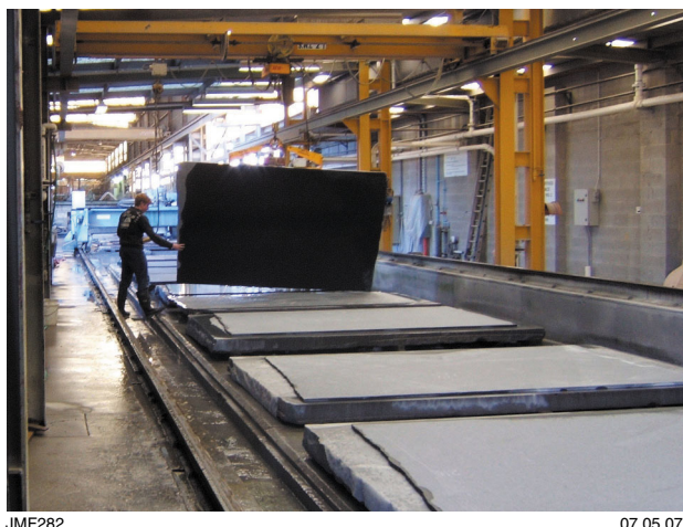
Figure 52. An overhead gantry crane lifts a cut slab onto a polishing line (photo courtesy Tillett Natural Stone Industries)
