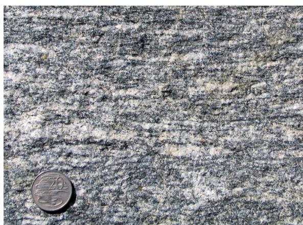
Figure 105. Detail of layered biotite monzogranite gneiss present at Roelands quarry
