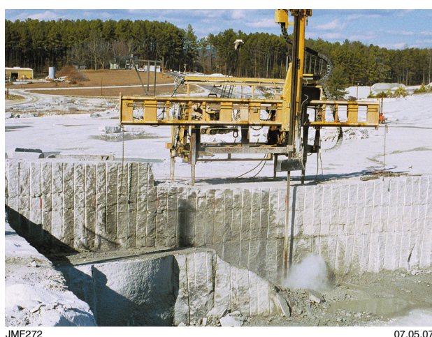
Figure 42. A high-pressure water jet cutting a vertical slot (76 mm wide) in granite (photo courtesy North Carolina Geological Survey)
