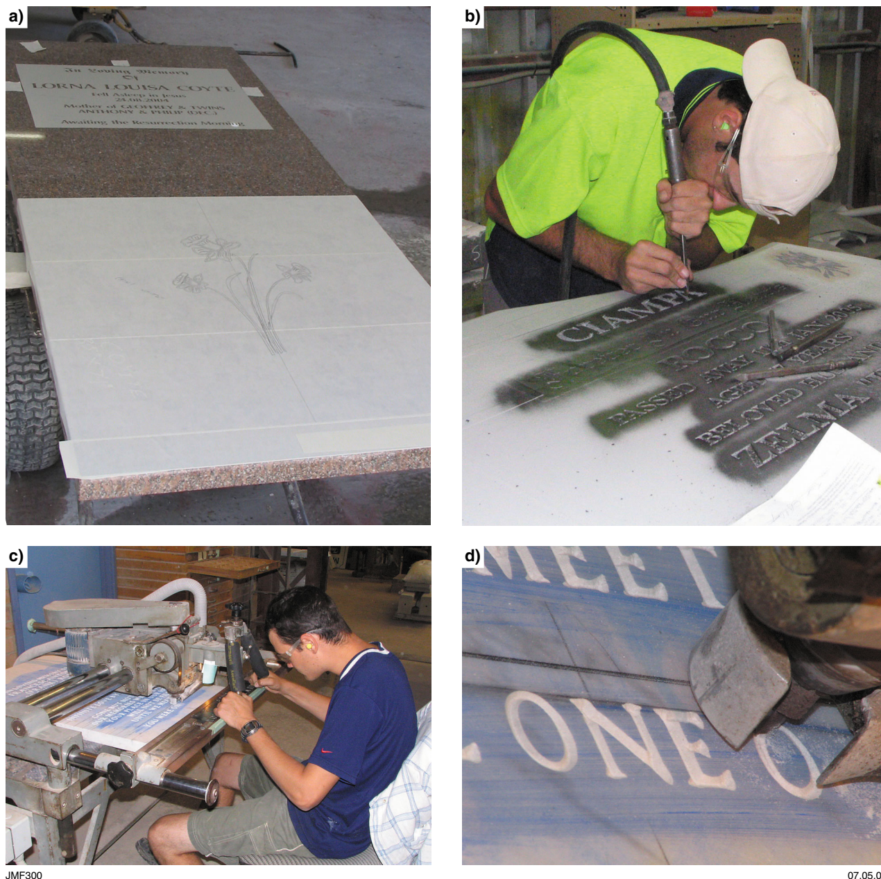
Figure 71. The stone engraving process: a) lettering template and floral design applied to a granite slab; b) engraver using a power chisel to cut stone lettering using an overlying template; c) operator using a pantograph machine to inscribe lettering onto a marble slab; d) detail of the engraving head cutting lettering into the marble surface
