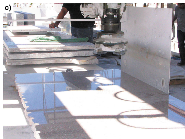
Figure 70. Operations in a stonemason's yard: a) block of red granite sawn into thick slabs by a blocksaw; b) stonemason welding a hand chisel to shape red granite blocks; c) granite slab after polishing by a single-head bridge polisher; d) bridge saw cutting component parts for a monument from a granite slab
