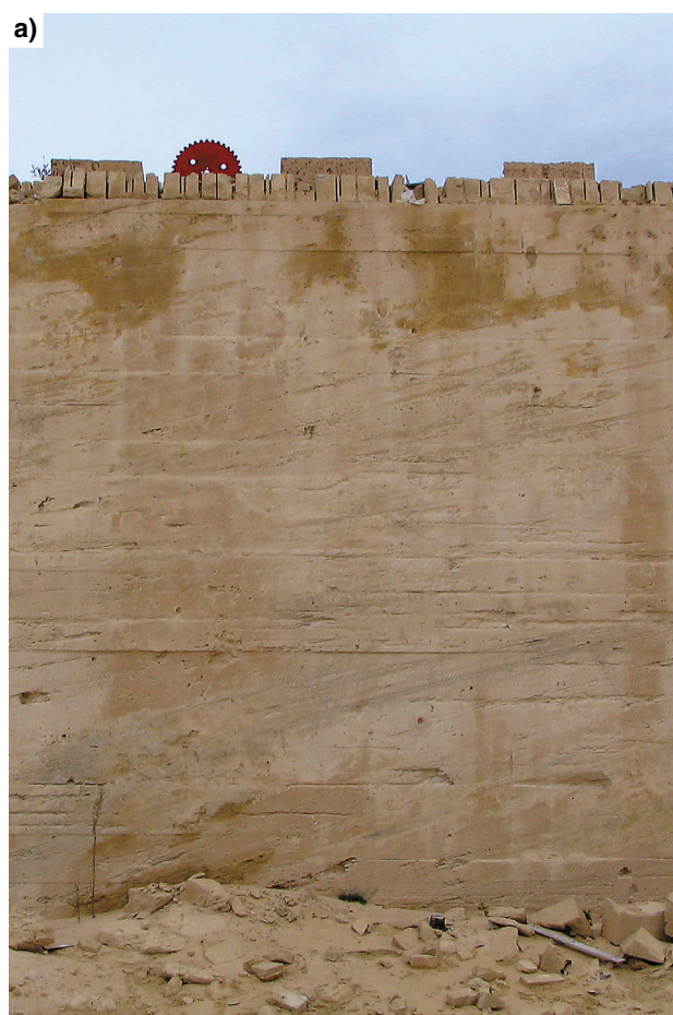
Figure 147. Tamala Limestone from Moore River: a) a six metre-high wall of massive, pale brown, crossbedded calcarenite in the Moore River block quarry; b) Moore River limestone bricks and blocks used in archways and as column cladding in a contemporary Italian-style villa (photo (b) courtesy Limestone Resources Australia, © Discovering Stone, 2006)
