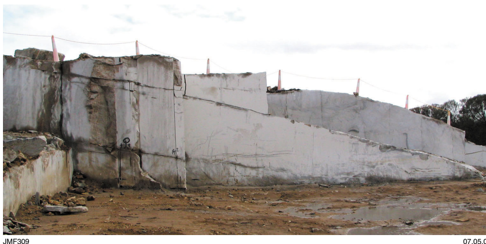
Figure 86. Austral Juperana granite gneiss quarry showing clean-cut, diamond-sawn block removal. Note primary block thickness (1.5–4.0 m) determined by subhorizontal unloading joint spacing
