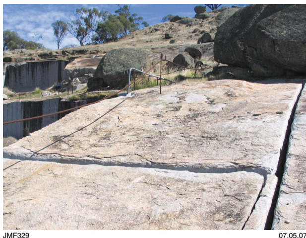
Figure 116. Large, primary blocks of quartz monzodiorite present in the Gwambygine quarry. Here, a thermal lance has been used to detach blocks from the quarry wall
