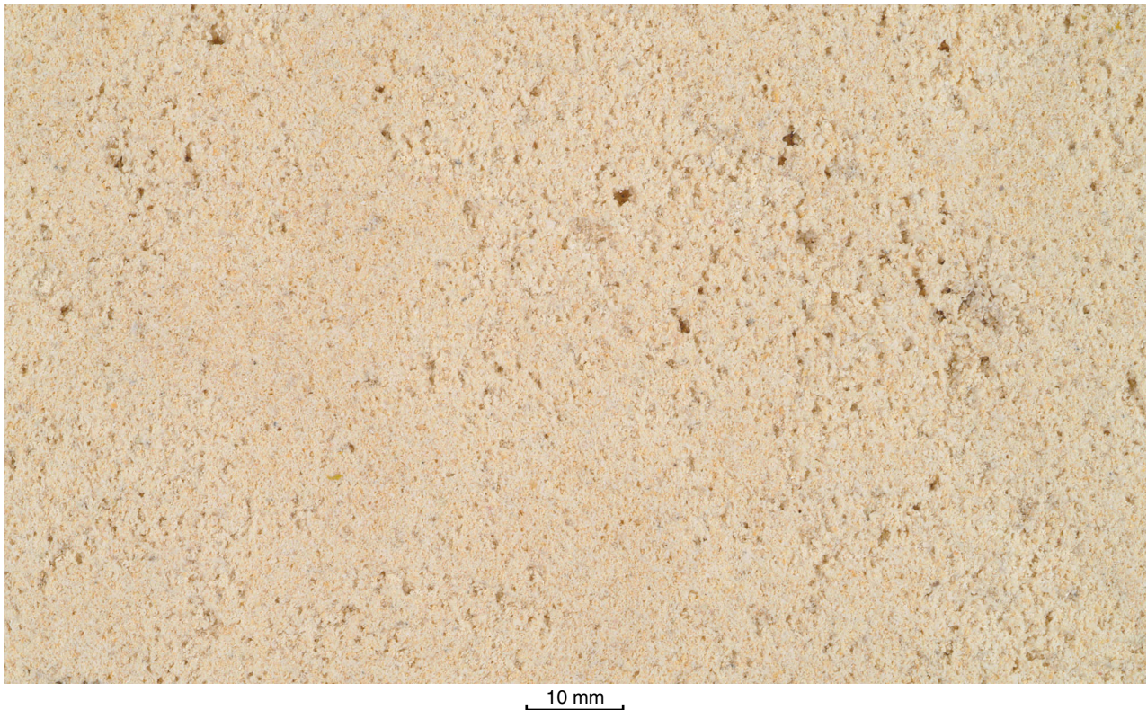
Appendix 3.30. Tamala Limestone: cream to pale brown, massive, porous, microfossiliferous limestone. A typical example of high-grade limestone building block material from the Carabooda–Nowergup area, Wattle Avenue quarry, Nowergup
