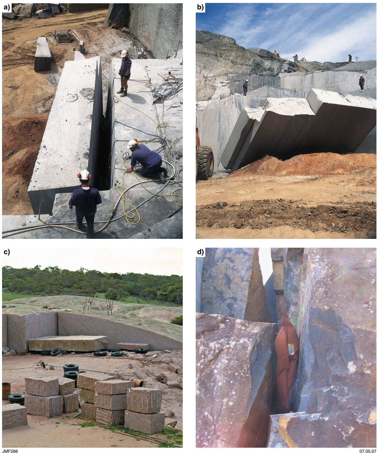
Figure 35. Tertiary block wedging and toppling: a) wedging completed with a block of black granite about to topple; b) black granite slab toppling onto a pile of soft earth; c) Block of red granite (at centre) toppled onto a pile of rubber tyres; d) pneumatic air bladder in position for wedging process (photos (a) and (b) courtesy Granites of Australia, photo (c) courtesy PIRSA)
