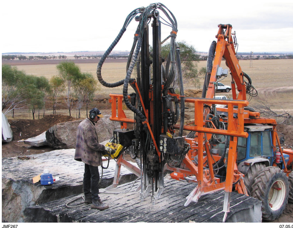
Figure 36. Tractor-mounted hydraulic boom arm supporting a rail-guided twin percussion drill rig at Austral Waterfall quarry near Bruce Rock
