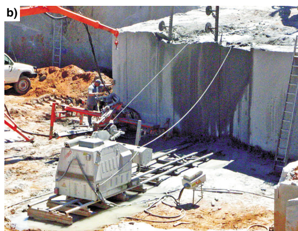
Figure 40. Diamond wire sawing operations: a) schematic diagram showing the operation of a diamond wire saw (modified from Smith, 1999); b) diamond wire saw cutting blocks of black granite
