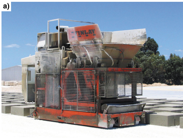
Figure 69. Batch making reconstituted limestone blocks: a) a mobile batching machine in operation; b) a newly formed set of reconstituted blocks, 1.0 m in length
