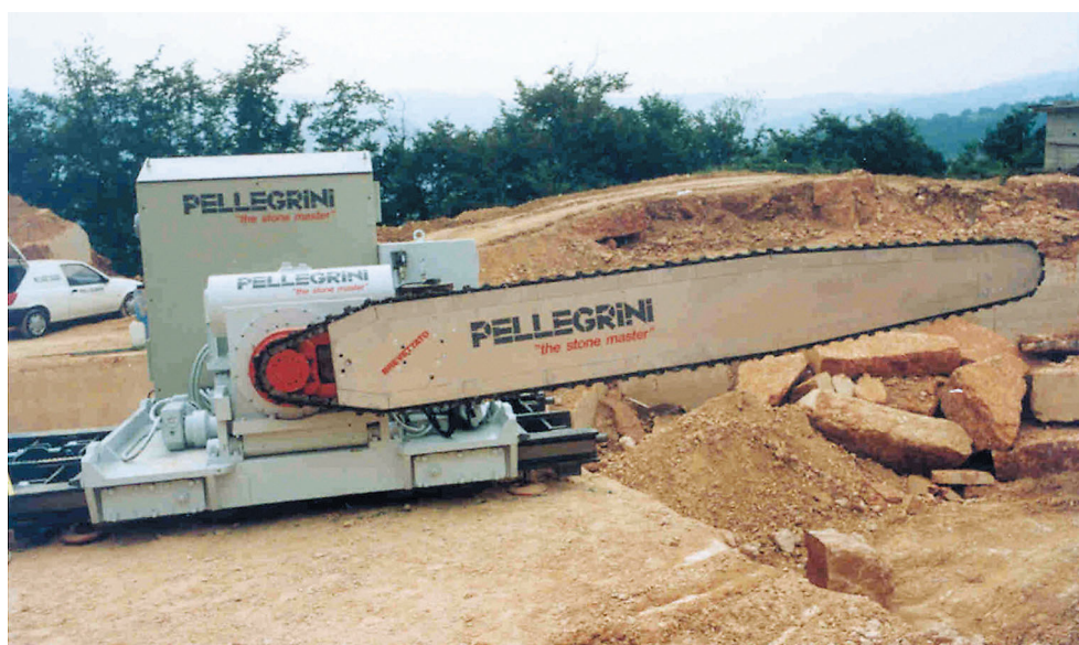
Figure 46. Electric-powered quarry saw fitted with a diamond impregnated cutting belt. The blade is approximately 2 m in length (photo courtesy Electrolux Construction Products Australia)
