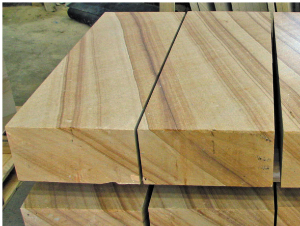
Figure 59. Large sandstone blocks rubbed to remove saw marks (block length about 1.0 m)
