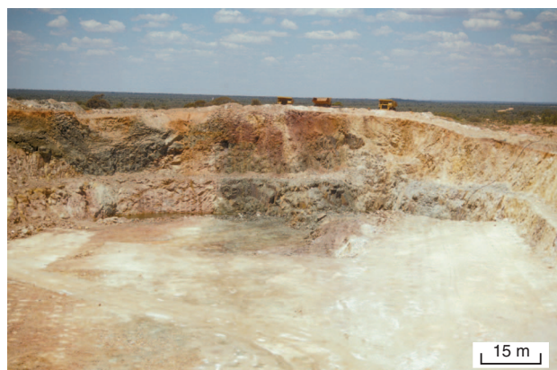
Figure 1.6. Gordon Sirdar openpit mine, looking south. The dark unit in the centre of the pit wall is the mineralized metamorphosed hyaloclastite unit. Gold associated with disseminated and veinlet pyrite was mined mainly from the contact zones of this unit
